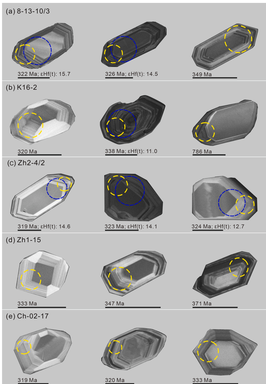
Fig. 3. Representative CL images of analyzed zircon grains, in which U–Pb ages and \epsilon_{\text{Hf}}(t) values are illustrated. Analyzed spots for U–Pb dating and Hf isotope analysis are indicated by yellow and blue circles, respectively. The black line below each zircon image is for scale (50 \mu\text{m} ). (For interpretation of the references to colour in this figure legend, the reader is referred to the web version of this article.)
